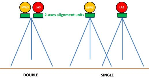
Figure 6: Mounting options for the combined OMS system.
