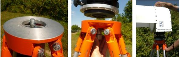
Figure 16: Fasten center bolt to mount RPG-MWSC-160 units on a tripod (single configuration).
