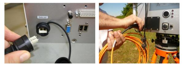
Figure 21: Setting up the fibre-optical cable for data transfer.
