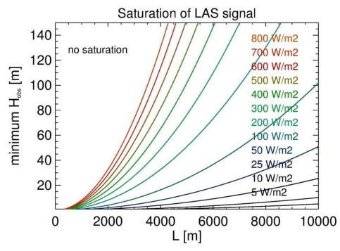
Figure 13: Saturation of the LAS signal in dependence of the observed sensible heat fluxes (T=300 K, RH=80%, p=1013.25 hPa), saturation criterion from Ochs and Wilson, 1993 [1].
