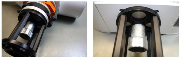
Figure 18: Mounting the height adaptors for LAS transmitter and receiver.
