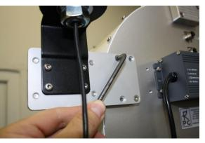
Figure 11: Mounting the GPS clock to the RPG-MWSC-160 receiver. The mounting plate can either be attached to the left or right side of the receiver housing.
