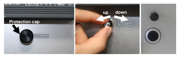
Figure 27: Remove protection cap on transmitter rear panel to adjust output power level.
