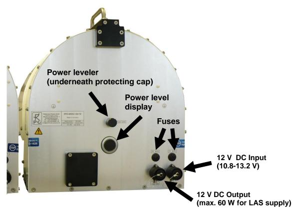
Figure 3: Rear view of the RPG-MWSC-160 transmitter.
