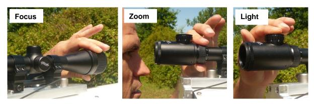
Figure 25: Adjustment of the MWS/LAS alignment telescopes.
