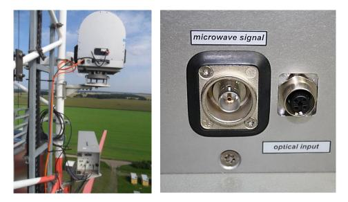
Figure 19: Left: OMS transmitters mounted on a measurement tower in Lindenberg, Germany. Right: BNC connector (left) to read the RPG-MWSC-160 detector voltage (only for diagnosis).
