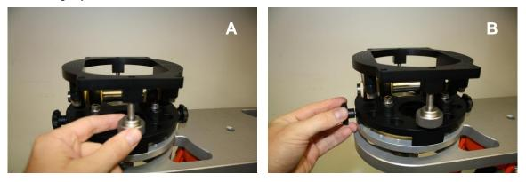
Figure 23: RPG-MWSC-160 alignment units allow adjustment of elevation (A) and azimuth (B) angle.
